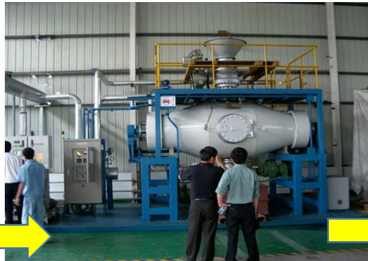
② Subcritical Water Processing (180°C/15atm@20-30min.)
